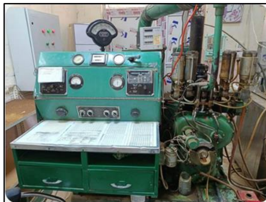
Fig. 5 Single cylinder –test engine assembly for RON measurements.
