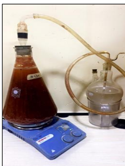
Fig. 1 The designed incubator designed to conduct anaerobic fermentation reactions.
